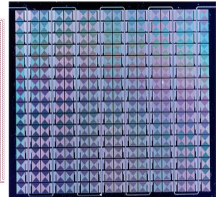
16 $\times$ 16 array of such pixels coupled to one microwave feedline
