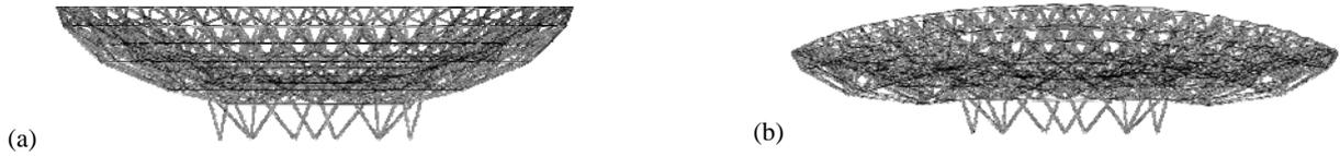
Fig. 15. Deformation due to gravity in Case 0 degree (Scheme 2) (a) Initial state (b) deformed state
