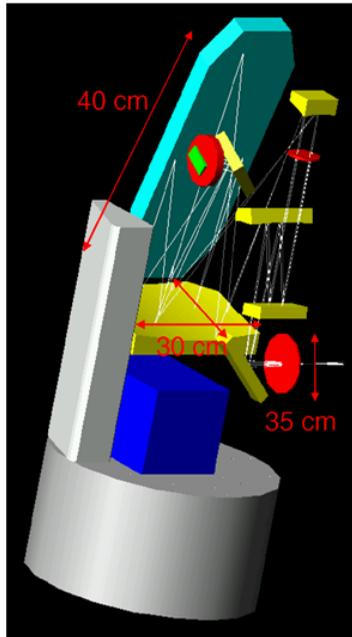
CCAT will utilize both wide field imagers and spectrometers. Shown is the ZEUS spectrometer, built by Cornell astronomers and very similar to concepts proposed for use with CCAT. JPL and Caltech also have plans and concepts for first light instruments which allow CCAT to reach its full potential very quickly after first light.
