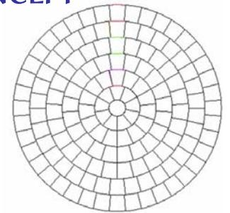
The CCAT primary mirror will be made up of multiple segments. The design shown above requires 145 panels but only six different types. This suggests the use of a replication technique which can yield substantial savings over making each panel to the requires precision.
